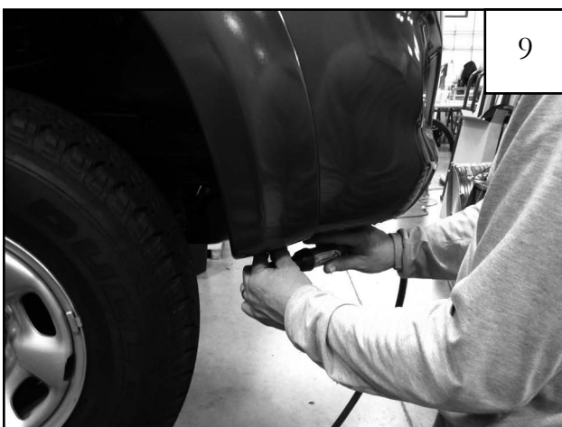
Remove 2 factory screws from under front bumper.
