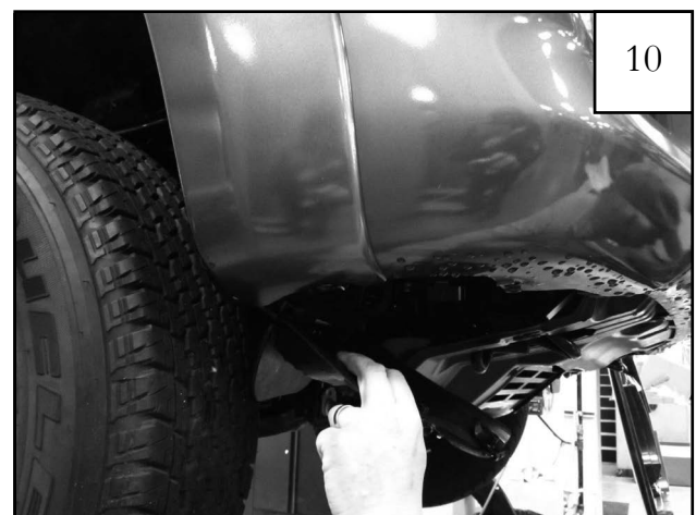
Pull down bumper cover and splash shield.
