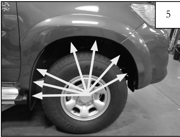
Remove seven factory screws from the fender lip. Save screws for reinstallation. Remove flare by pulling part away from side of vehicle.
