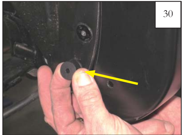
Install supplied grommet (GR1-0001) into factory hole.
