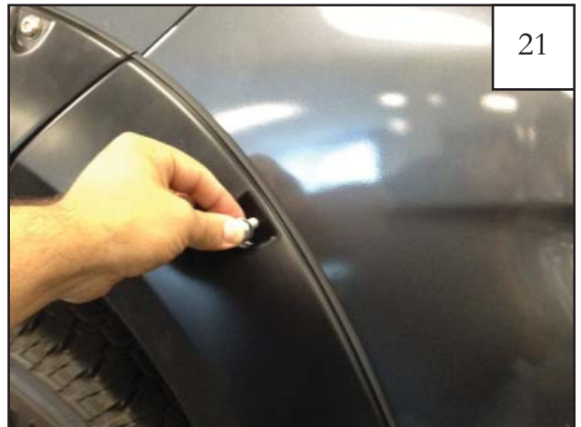
Slide a supplied .320 SS Washer (WA1-0012) onto a SS Torx Screw (SW1-0041). Inserting screws through holes drilled in bumper in step 20.
