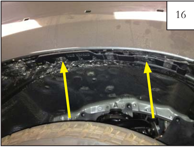
Line the bracket up with the two uppermost factory holes in the fender. Use two factory screws to install bracket onto fender.
