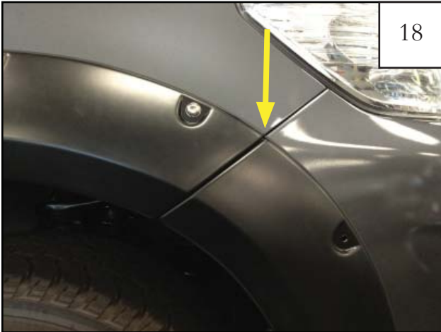
Make sure bumper piece is aligned with the style line.
